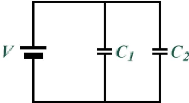
Suppose  $C_1$  was  $3 \times 10^{-9}F$  and  $C_2$  was  $2.3 \times 10^{-10}F$ . What is the total capacitance?
