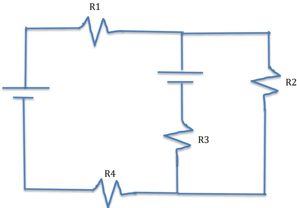
The battery on the left is 15V and the battery on the right is 6V.  $R_1=10\text{ohms}$ ,  $R_2=3\text{ohms}$ ,  $R_3=6\text{ohms}$ , and  $R_4=9\text{ohms}$ .
