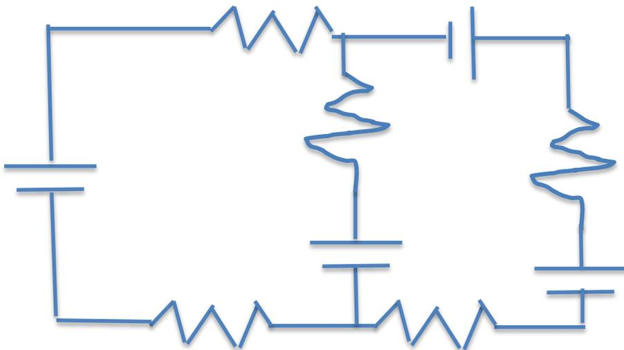
In the circuit above  $V_1 = 12.1\text{V}$ ,  $V_2 = 5.9\text{V}$ ,  $V_3 = 17.2\text{V}$ , and  $V_4 = 3.2\text{V}$ .  $V_1$  was used to guess the current direction.  $I = 3.5\text{A}$  and travels clockwise from battery 1, and
